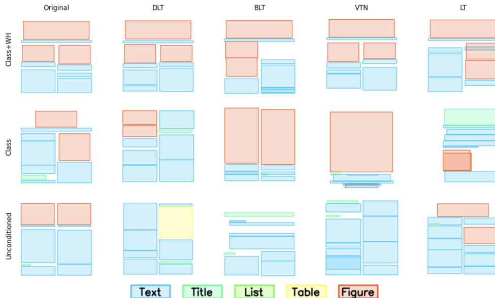
Figure 4: Qualitative comparison of generated layouts between all tested methods on PubLayNet dataset with the three tested conditioning settings.
