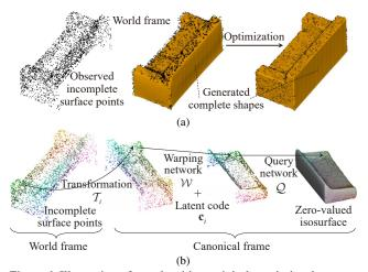
Figure 6. Illustration of our algorithm to jointly optimize the transformation and latent code. (a) In the world frame, the generated shape is better aligned to the observed surface points thanks to our optimization. (b) Surface points in the world frame correspond to the zero-valued isosurface of SDF in the canonical frame.
