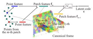
Figure 4. Illustration of our latent code prediction based on *intrainstance* information. Given a point set of an instance in the canonical frame, we first extract the feature of each point. Then we segment a point set into several patches, and extract the feature of each patch based on the features of points belonging to this patch. Finally, we aggregate features of patches to obtain a latent code.
