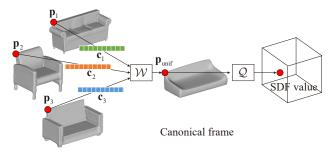
Figure 3. Illustration of deep implicit template. Position warping sub-network W takes different latent codes  $\{\mathbf{c}_i\}_{i=1}^N$  as input and maps different positions  $\{\mathbf{p}_i\}_{i=1}^N$  into a unified position  $\mathbf{p}_{unif}$ . SDF query sub-network Q predicts SDF value of the position  $\mathbf{p}_{unif}$ .
