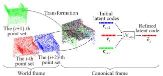
Figure 5. Illustration of our latent code prediction based on *inter-instance* information. Three input point sets in the world frame correspond to similar one-seat sofas. We transform them into the canonical frame and predict their initial latent codes separately. Then we refine the latent code of the *i*-th instance by integrating the initial codes of this instance and its neighbors.
