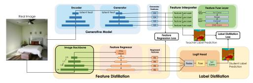
Figure 3. **DreamTeacher architecture**: Feature regression module (FR) maps and fuses multi-scale features of a (CNN) image backbone. We supervise FR with features from the generator's decoding network. We optionally add a *feature interpreter* [82] to the generator to train a task head with supervised labels – used to supervise the image backbone with label distillation loss.
