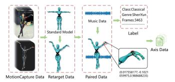
Figure 2. FineDance acquisition process. We capture the dancers' motions with the Vicon optical motion capture system. Then engineers retarget it to a standard skeleton in MotionBuilder. Dancers manually align the music with the dance motions and extract the skeletal information of the dance in Blender.
