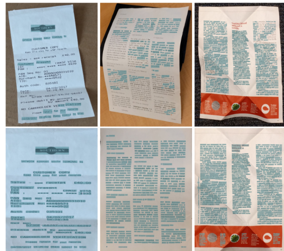
Figure 1. Compared with the text results using Tesseract [32] as OCR engine. Row 1: distorted images. Row 2: rectified by our method. We use color to highlight the detected text boxes.
