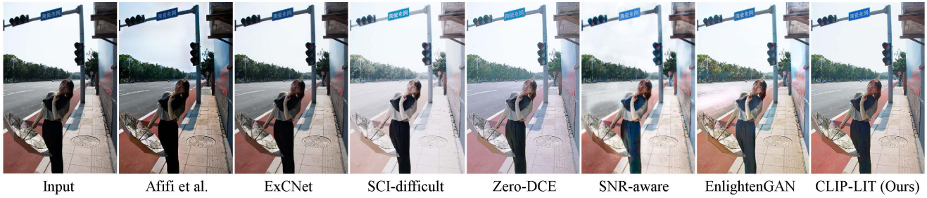
Figure 3: Visual comparison between our method and the state-of-the-art light enhancement methods, including exposure correction method (Afifi et al. [1]), backlit enhancement method (ExCNet [32]), low-light image enhancement methods (SCI [22], Zero-DCE [10], SNR-aware [29], EnlightenGAN [11]). Our method effectively enhances the backlit image without introducing artifacts and over-/under-enhancement.
