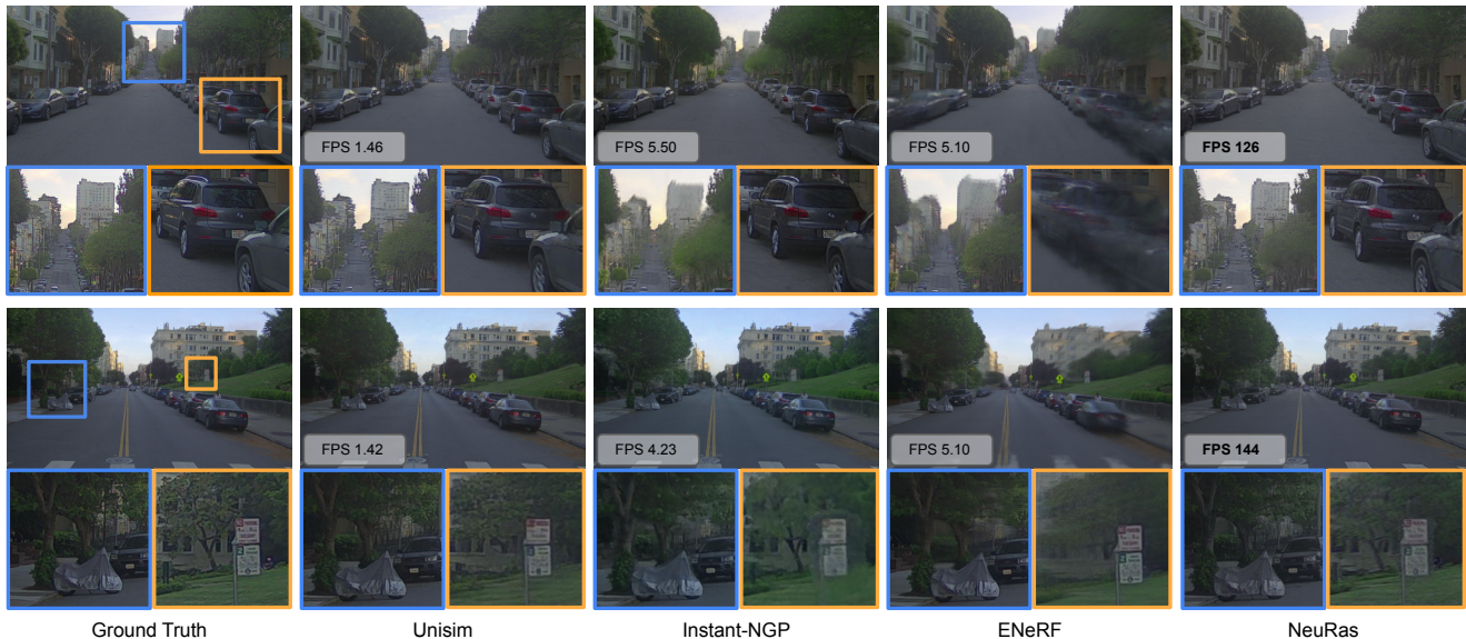
Figure 5. Qualitative results on driving scenes. Compared to existing novel view synthesis approaches, NeuRas produces competitive realism and achieves real-time rendering ( > 100 FPS).
