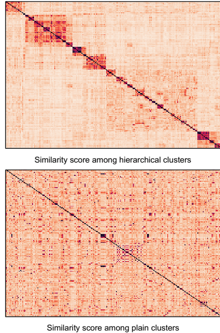
Figure 3. Visualization of the similarity scores between clusters for (Top) hierarchical clusters and (Bottom) plain clusters. The hierarchical clusters have a well-defined structure whereas the plain clusters appear nearly arbitrary. We construct the hierarchy in hyperbolic space based on the similarities between the hierarchical clusters.
