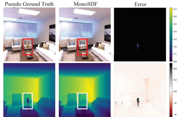
Figure 4. Illustration of failure cases of state-of-the-arts. Even though applying the perfect pseudo ground-truth geometry to supervise the model, existing room-level reconstruction methods like [36] can still fail to resolve accurate 3D structures.
