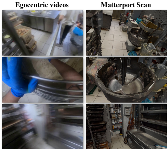
Figure 3. Egocentric Videos and Matterport Scan. We show illustrations of the domain gap between Matterport Scan and real scenes. Matterport Scan may have different illumination, scene appearance, and missing/low-quality scans. Egocentric videos are usually dynamic, free of view (FOV), and have fast motion blur, bringing great challenges for 3D reconstruction and localization.
