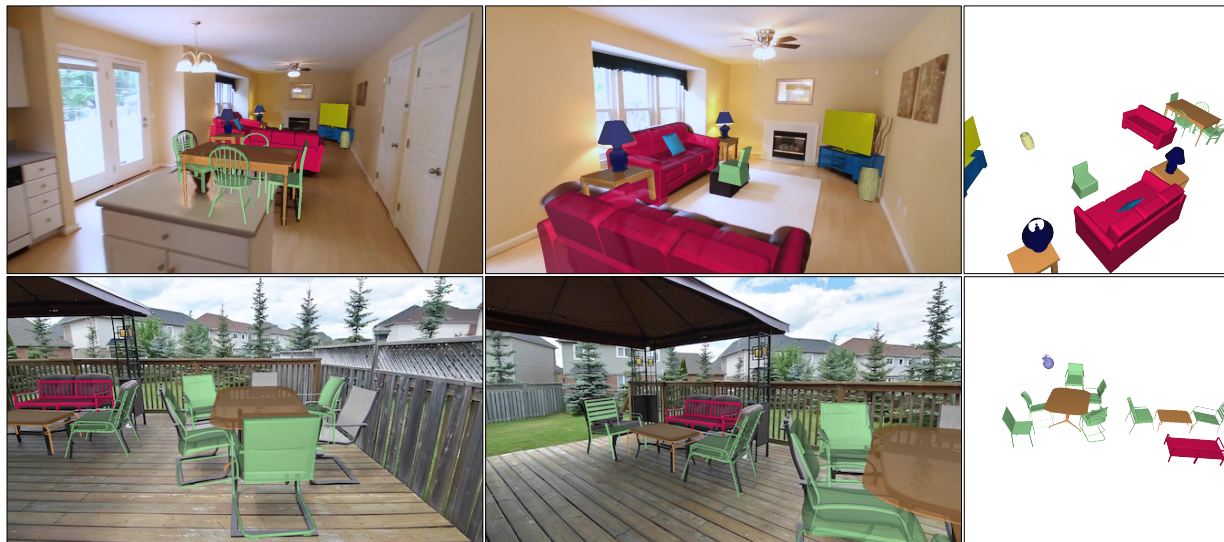
Figure 1. Example annotations of the CAD-Estate dataset. We create globally consistent 3D representations from RGB videos, by retrieving CAD models and estimating their poses. We visualize them by overlaying them on the video frames (left, mid), and from a top-view (right).
