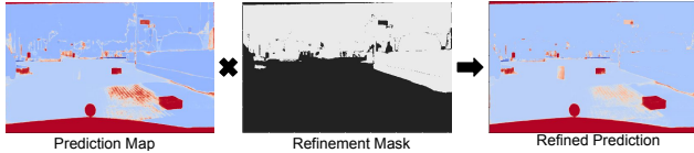
Figure 4: Mask Refinement Illustration: To obtain the refined prediction, we multiply the prediction map with a refinement mask that is built by assigning zero anomaly scores for pixels that are categorized as “stuff”, except for the “road”. The refinement eliminates many false positives at the boundary of objects and in the background. The region to be masked is white in the refinement mask.
