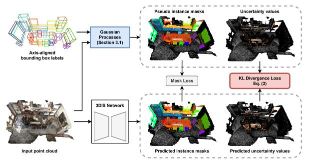
Figure 2: **Overall architecture of our approach**. GaPro is a two-step approach consisting of leveraging Gaussian Processes to generate pseudo instance masks and their uncertainty values, and training a 3DIS network to match its prediction against these pseudo labels with a new KL divergence loss along with the mask loss.
