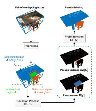
Figure 3: **Our Gaussian Process**. For each pair of overlapping boxes, the determined and undetermined regions are identified and taken as input into a Gaussian Process to produce pseudo mean and variance values. Then the Probit function is utilized to output the posterior Bernoulli distribution as pseudo labels.
