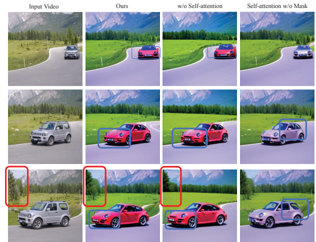
Figure 9. Ablation study of blended self-attention. Without self-attention fusion, the generated video can not preserve the details of input videos (e.g., fence, trees, and car identity). If we replace full self-attention without a spatial mask, the structure of the original jeep misleads the generation of the Porsche car.
