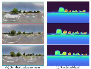
Figure 1. Sat2Density trains with a collection of satellite-ground image pairs, without depth, or multi-view supervision. Our 3d GAN enables the synthesis of scenes conditioned on a satellite image, producing multi-view-consistent ground-view renderings and geometry. *Please see the project page for more videos*.
