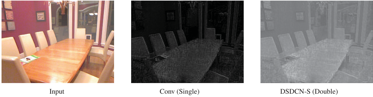
Figure 8: Comparison of feature map visualization for single-scale and multi-scale tokens. The design of multi-scale and multi-branch can capture more powerful features.
