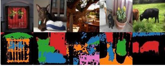
Figure 3: Visualizations of bottom-up grouping by CLIPpy. Each color represents one grouping learned on a given image.
