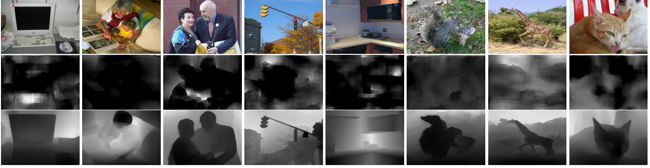
Figure 5. Failure cases reported by [27]. The second row shows “noisy” depth maps from [27] (VG-Depth.v1). The bottom row represents the improved depth maps used in VETO (VG-Depth.v2), generated using the monocular depth estimator of [45].
