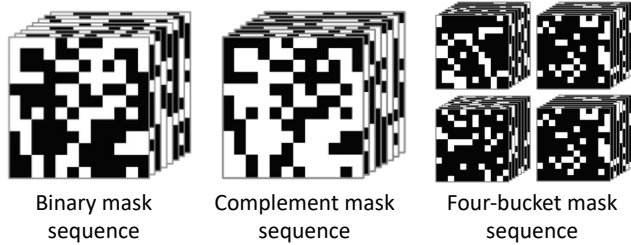
Figure 3: Modulating masks for video compressive sensing. (left) A single VCS measurement temporally compresses a sequence of frames using binary random masks. (center) Two-bucket cameras capture an additional measurement by using the complementary mask sequence. (right) We propose using multi-bucket captures by randomly choosing an active bucket for each frame. Both two-bucket and multi-bucket captures have 100% light efficiency. All masks are visualized here for 16 \times 16 pixels.
