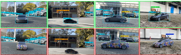
Figure 9: Real-world evaluation using two scaled cars. The upper row is the normal car model, while the bottom row is the adversarial camouflaged car model. Zoom for detail.
