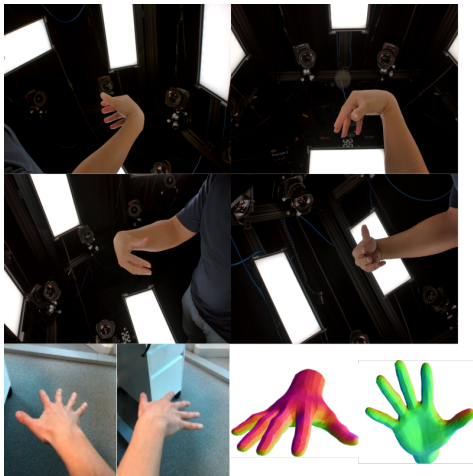
Figure 8: Training examples of our real dataset ( top ) and 3D hand mesh estimation results on in-the-wild image ( bottom ). The resulting mesh contains 3745 vertices.
