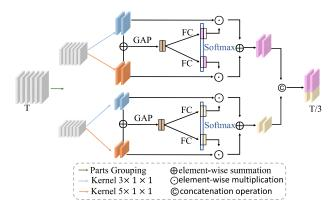
Figure 3: The detailed structure of the frame-level temporal aggregation (FTA). For simplicity, we omit the channel dimension C.
