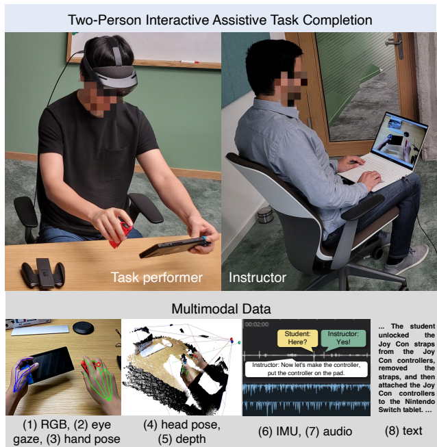
Figure 1: HoloAssist features a two-person interactive assistive task completion setting. The task performer wears an AR device and completes the tasks while the captured data is streamed over the network to a remote instructor watching it on the laptop. The instructor provides verbal guidance to the student. HoloAssist includes seven modalities captured live and human annotated text descriptions as the 8th modality.
