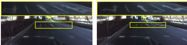
Figure 7: Fused frame sequence with the homography transformation between the frame pairs. The road surface normal estimated with feature representation enables more accurate homography transformation than with RGB information, resulting in better alignment of road lines and markings across frames.
