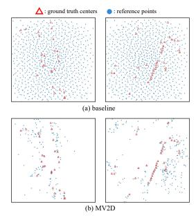
Figure 6. Illustration of different kinds of object queries. The top row (a) represents the *baseline* method (fixed object queries) and the bottom row (b) represents our method (generated object queries). We visualize ground truth center locations and the reference points in BEV space. The samples are taken from nuScenes *val* set. We suggest readers view this figure by zooming in.
