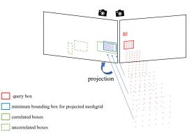
Figure 4. Illustration of relevant region selection. Each query box generates a discretized camera frustum from 3D meshgrid. The camera frustum is then projected to another view's pixel coordinate to calculate a minimum bounding box. Then the relevant box is selected based on the overlap with the minimum bounding box.
