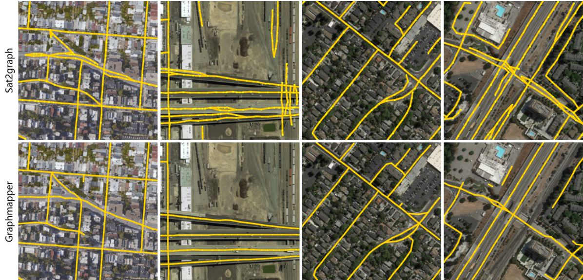
Figure 3: Qualitative result of road mapping on City-Scale dataset. Top row is from Sat2Graph, bottom row is our method. Our method shows to generate improved road topology compared to Sat2Graph in various scenarios.
