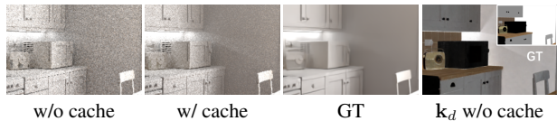
Figure 5: Diffuse radiance cache from \mathbf{L}' helps reduce variance and error for shading estimation (2nd image). Without it, sampling the tiny emitters below the cabinet will be difficult (1st image), which leads to incorrect shading and albedo (4th image).
