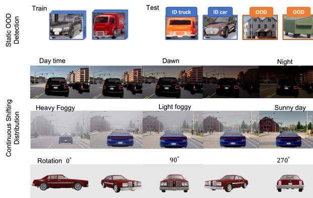
Figure 1: Difference between existing static OOD detection and a more realistic scenario of Continuously Adaptive OOD Detection (Problem 1) when test samples come from continuously shifting distribution, i.e., Definition 1.
