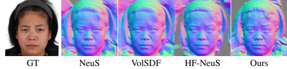
Figure 8. Our method is capable of reconstructing the geometry of the entire head, in particular providing better results in the hair region of human heads compared to other methods. This is due to the fine refinement of the SDF using the displacement field. Model: 429, 15 views.
