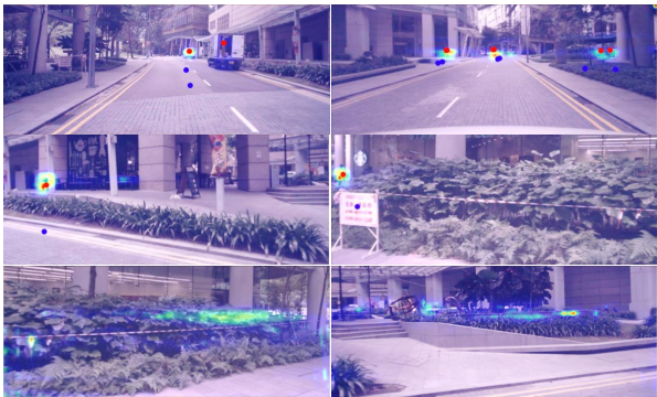
Figure 6: Visualization of attention maps on multi-view images. The blue points (●) are initial anchor points while red points (●) are the centers of box predictions. It shows that high response regions of attention maps mainly focus on the foreground objects, which are close to the anchor points.
