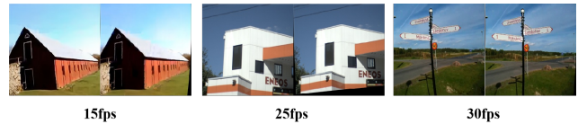
Figure 13. Correction on real RS images with different framerates. In each pair, the left is RS image and the right is corrected result, which shows the generalizability of the learned-bases.
