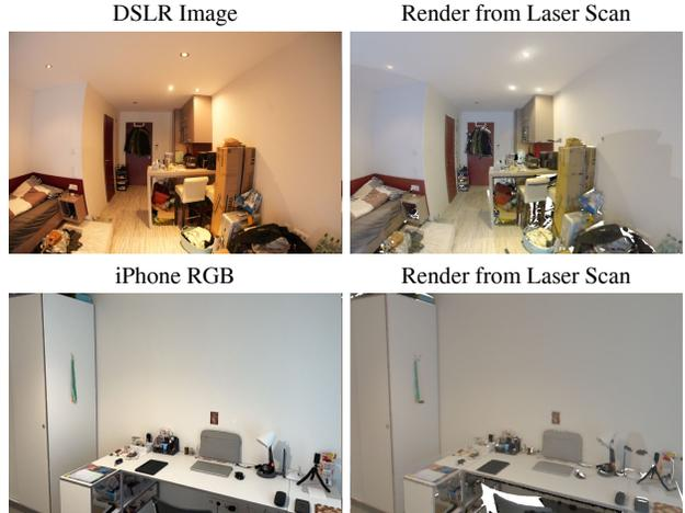
Figure 4: Examples of the alignment between DSLR, iPhone, and the scanner in ScanNet++. We obtain accurate alignment of all 3 sensors into the same coordinate system, empowering research across three modalities.
