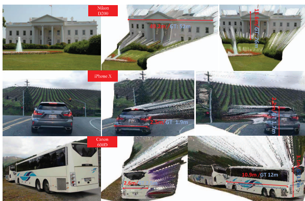
Figure 7 – Reconstruction of in-the-wild scenes. We collect several Flickr photos, which are captured by various cameras. With photos’ metadata, we reconstruct the 3D metric shape and measure structures’ sizes. Red and blue marks are ours and ground-truth sizes respectively.
