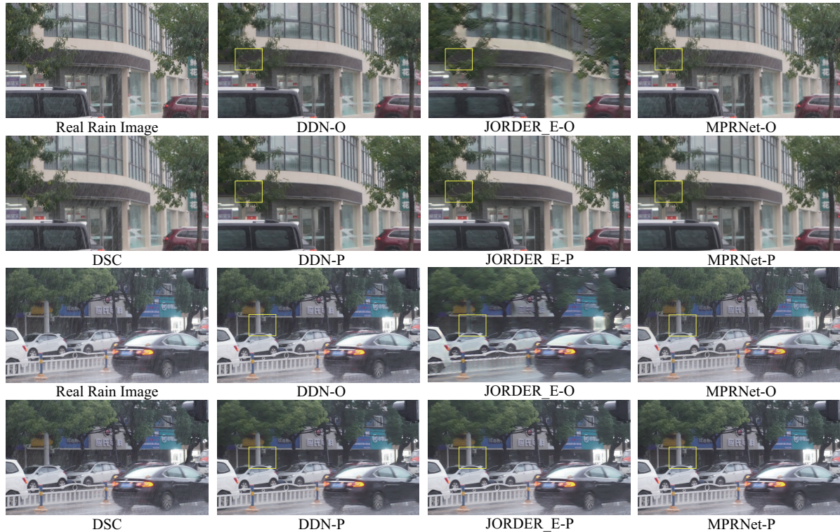
Figure 7: Performance comparison on the unpaired real rain FCRealRain, including rainy image, deraining result from DSC, and deep SOTAs trained on the original datasets SPA (1 st row) and generated dataset by PCGNet (2 nd row).
