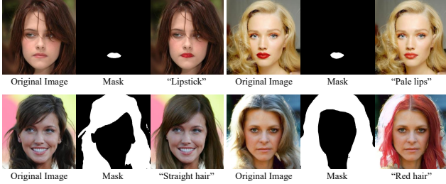
Figure 4: Practical usage of face parsing maps. We can limit the gradient of the energy function to update the image only in the target semantic region indicated by the mask so that other regions remain unchanged while editing.
