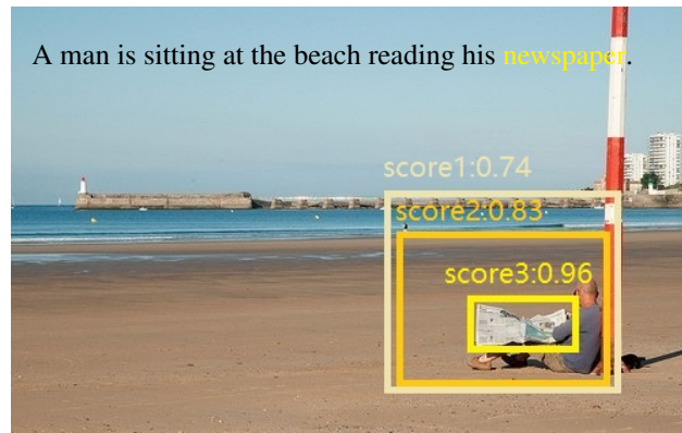
Figure 6. Illustration of the coarse-to-fine process of region adaptation. We also show the matching score between the regions and counterpart words. Note that each region at different levels in the region adaptor has independent scaling and moving behavior in our implementation.
