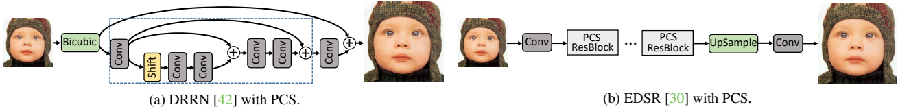
Figure 2: Schematic diagram of the PCS applied to the existing SR models. (a) DRRN [42] is a representative lightweight model with recursive structure, while (b) EDSR [30] is a typical largescale model with modularized residual learning. For EDSR [30], the PCS is embedded into each residual block for periodic feature enhancement. Please note that our PCS does not introduce extra parameters and computation other than negligible overhead for data movement.
