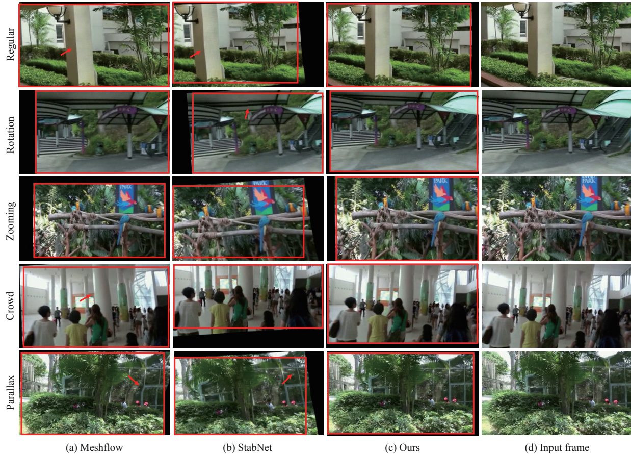
Figure 5. Qualitative comparisons with the online methods Meshflow [22] and StabNet [33]. We keep the original warped frames for comparison. The red boxes indicate the preserved frame content after cropping. The red arrows highlight the shear and distortion artifacts.
