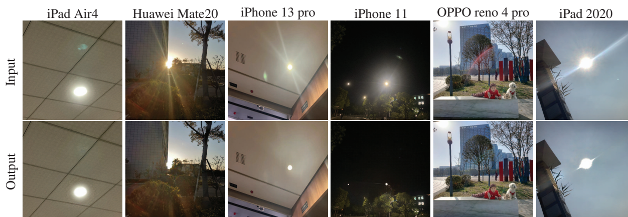
Figure 1. The proposed solution yields favorable results on the flare-corrupted images captured by various devices. The real and diverse flare-corrupted images are provided in our consumer electronics test dataset. The results are produced by the deep model U-Former trained using our solution that includes the new data synthesis pipeline and multiple light sources recovery strategy.
