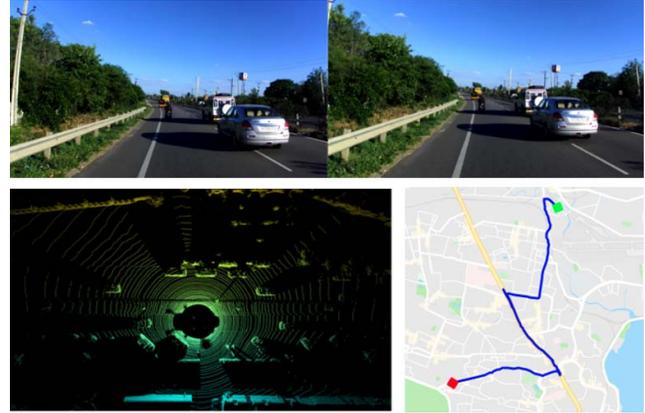
Figure 1. Visual representation of an example multimodal data. Top: RGB image from a stereo camera. Bottom: GPS coordinates plotted on a map and LiDAR pointclouds plotted in a 3D graph.
