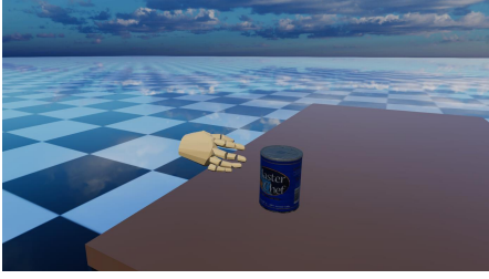
Figure 5. Physics Simulation. We create a controllable hand model and deploy it in the RaiSim physics-engine [7] to provide us with information about contacts and dynamics.
