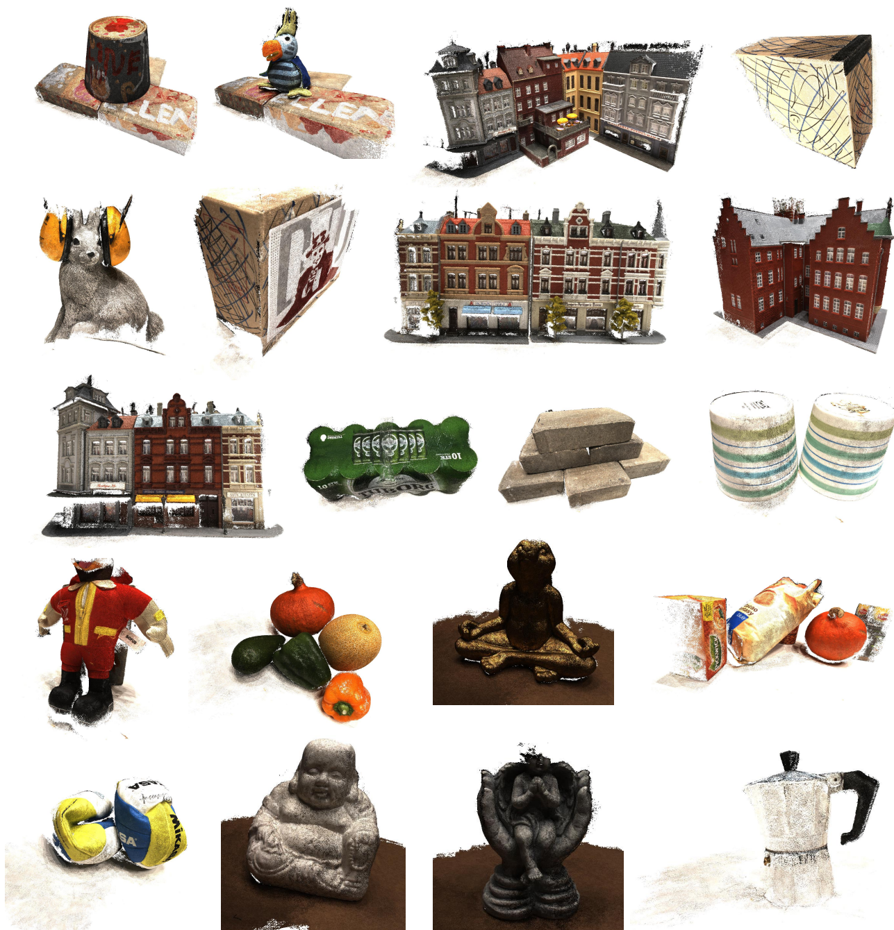
Figure 4. Point clouds of our method on DTU dataset [2].
