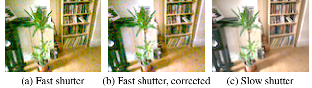
Figure 4. (a) Fast and (c) slow captures of the testyucca scene, with brightness normalized by shutter speed (heavily downsampled to minimize noise). These two images should match perfectly, but have a perceptible color difference due to the miscalibration documented in Section 4.4 and Figure 3. (b) In the center, we show a version of (a) with per-channel rescaling in the raw domain to match the global color balance of (c).
