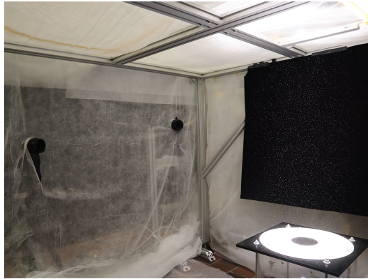
Figure 7. View of the experimental setup with two cameras and the vortex generator.
