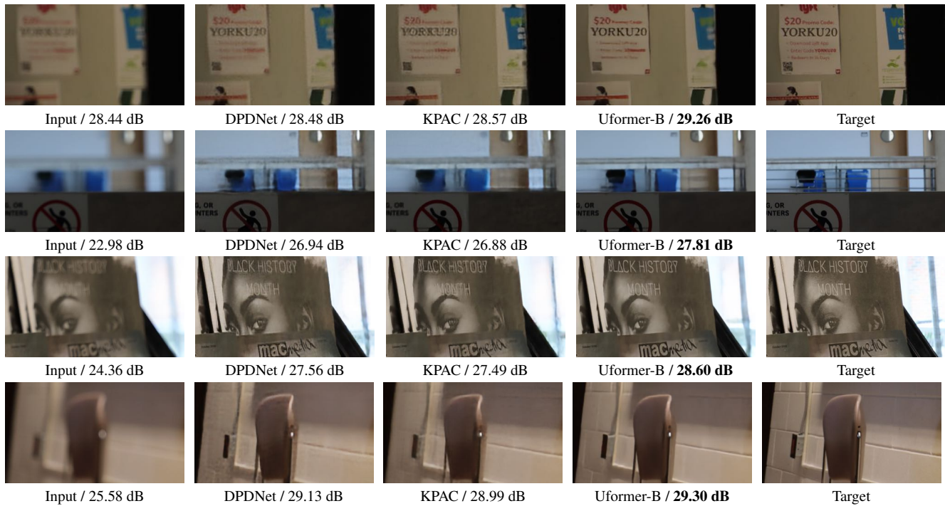
Figure D. More results on DPD [2] for image defocus deblurring. We report the performance of PSNR on the whole test image and show the zoomed region only for visual comparison.
