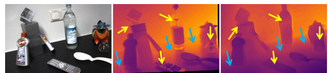
Figure 7. Sensor Fusion. Scene (left) with I-ToF depth (centre) and ToF+RGB Fusion [27] (right). Fusion can help to resolve some material induced artefacts (yellow) as well as MPI (blue).
