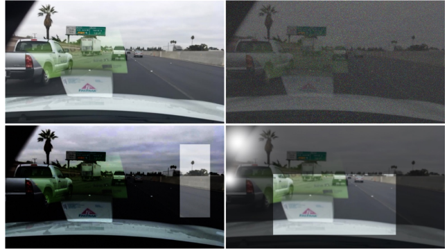
Figure 4. NightAug: Original image (top-left) and images with random augmentations from: gaussian blur, gamma correction, brightness, contrast, glare, gaussian noise and random cut-outs.
