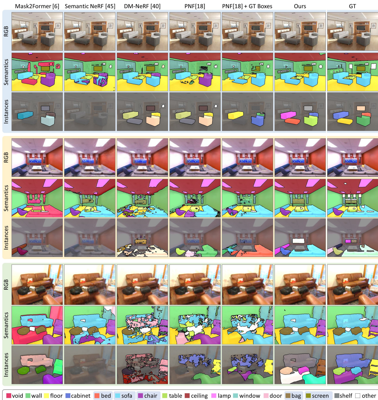
Figure 6. Novel views and their corresponding semantics and instances on Hypersim [29], Replica [34], and ScanNet [9] (top to bottom, respectively). Highlighted legend labels represent instanced ( thing ) classes. All 3D methods use the same posed RGB images and 2D machine-generated labels for training. PNF [18] additionally uses 3D bounding box predictions, while PNF + GT Boxes uses ground truth bounding boxes for instance classes. We outperform the state of the art, producing clean and consistent segmentation masks.
