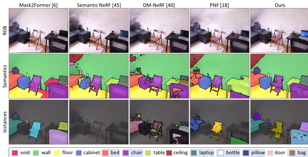
Figure 7. Novel views and their corresponding semantics and instances on in-the-wild room capture. Highlighted labels in the legend represent instanced ( thing ) classes. All 3D methods use the same posed RGB images and 2D machine-generated labels for training. PNF [18] additionally uses predictions from a 3D bounding box detector.
