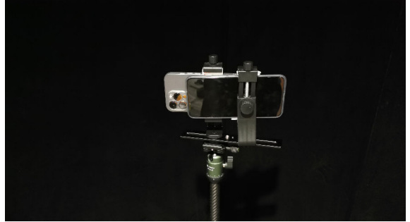
Figure A1. A close-up picture of our custom-built camera setup consisting of two smartphones mounted on a tripod.
