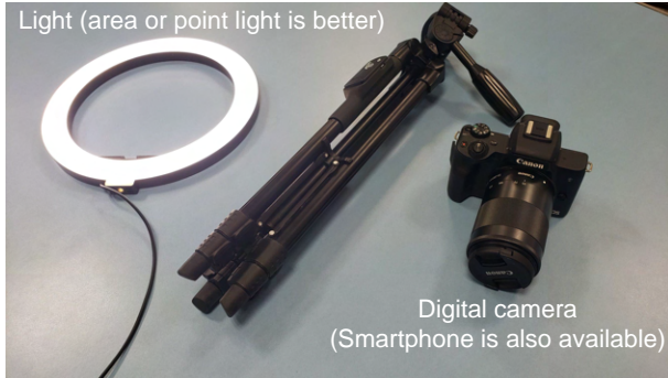
Figure 2. Our acquisition setup simply needs a movable light source and a camera.
